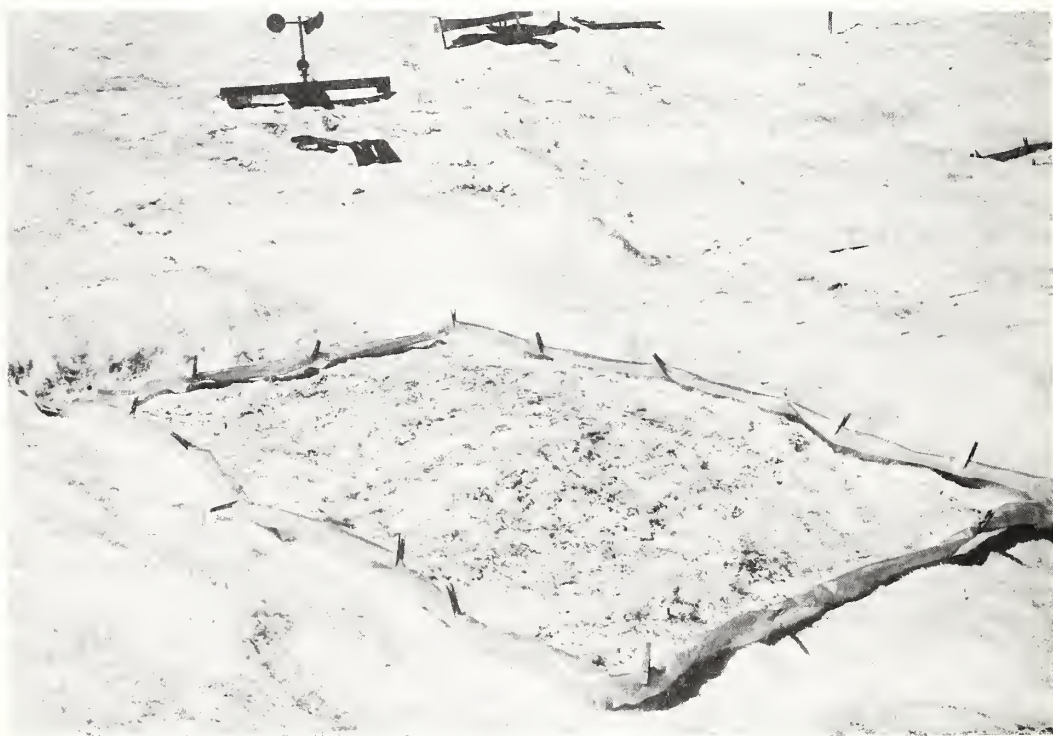
Figure W-1. --Tanks made of plastic sheeting were used to measure the net moisture exchange between the air and an alpine snowfield. They were filled with 4,860 pounds of snow. A plastic tube carried melt water to a container from which it could be poured for frequent weighing. At the end of the period the combined weight of the melt water and the remaining snow exceeded the original snow weight, indicating that more moisture was gained by condensation than was lost by evaporation. The net gain was 0.37 inch of water per week for one lysimeter and 0.29 inch per week for the other. Hence under the conditions that prevailed during this period, each acre of snow milked about 1,300 gallons of water a day from the air.
